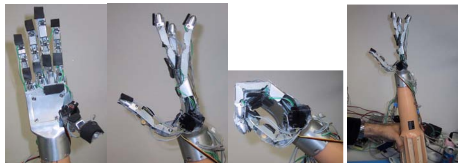
(a) Aluminum body of a finger part and a palm part (b) Whole products
