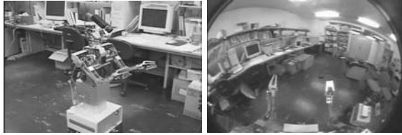
Fig. 13. Visuo-Motor Learning Experiment. Left: Outlook of the robot. Right: View from the robot's eye.
