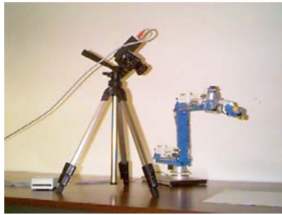
Fig. 2. The robot arm and stereovision system simulated in the experiments.
